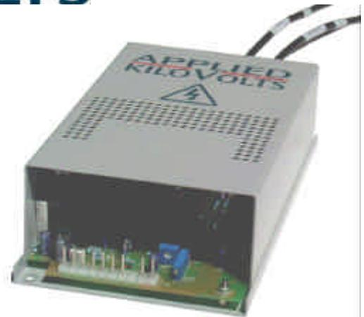
These power supplies, based on the standard HP series (data sheet HP Series refers) are intended to power imaging detectors. They give 0 to +3.5 kV and can be floated on voltages up to  $\pm 2.5$  kV (HFxx2.5),  $\pm 10$  kV (HFxx010),  $\pm 20$  kV (HFxx020) &  $\pm 30$  kV (HFxx030) and use differential feedback techniques to allow the **24 volt power, control and monitor** signals to be at **ground potential**.
